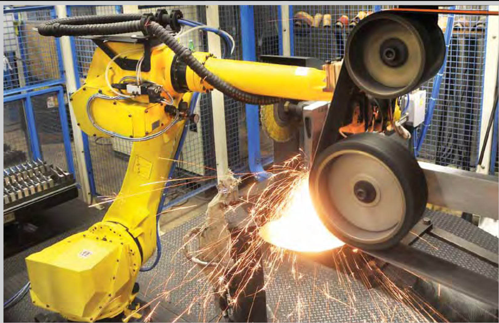
Purchased in Italy in 2009, this robot can work 24 / 7 and sharpen hundreds of tool heads a day.
