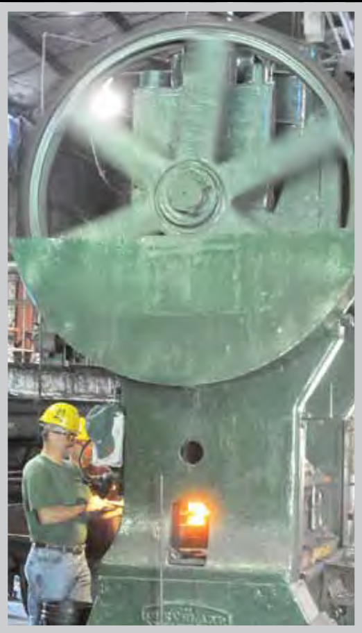
Nicky McLamb operates a cold press.
