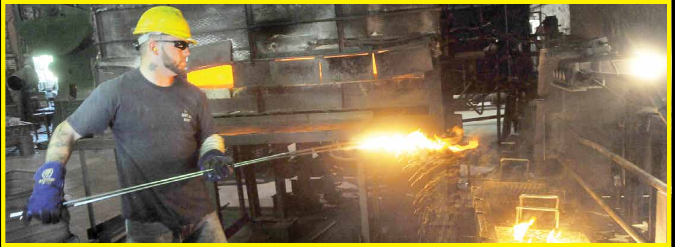
Raeford Jones heat treats a red-hot shovel head from the furnace by immersing it in a quenching solution.
