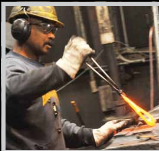
Williams Spears "upsets" (punches out) the eye of an ax head.
