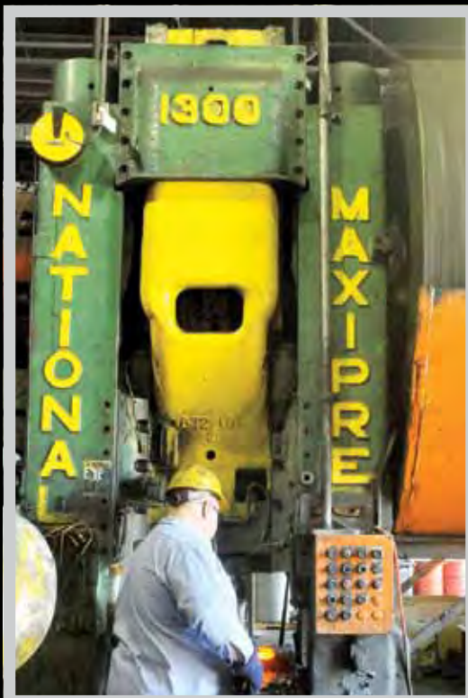
Yogi Simmons forges sledgehammer heads on a massive flywheel press.
