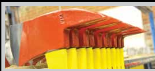
Williams Spears "upsets" (punches out) the eye of an ax head.
