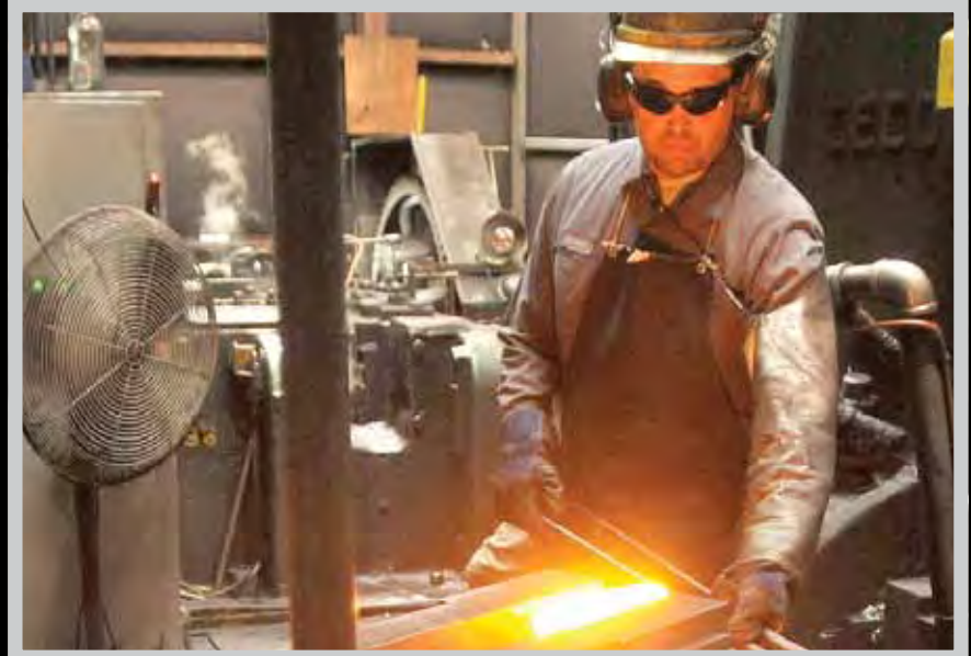
Richard Robinson gets a red-hot billet from an induction furnace.
